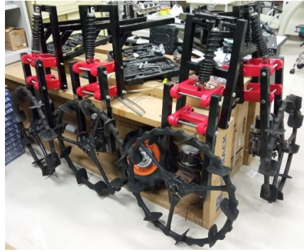
Figure 6. The wheel frame of the rice farming applicator robot
