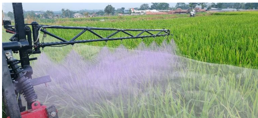
Figure 10. Liquid distribution pattern synchronized with forward speed
