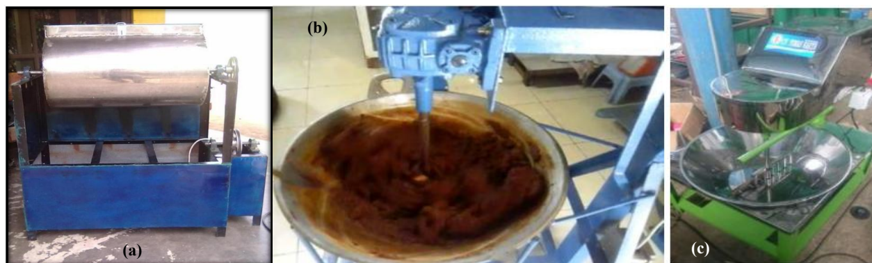
Figure 3. Different machine to crystallize palm sugar: (a) Tubular-type palm sugar ( Yunanto, 2012 ); (b) Open-pan palm sugar stirrer ( Pardede, 2018 ); (c) Sap cooking machine ( Indrawati et al. , 2020 ).
