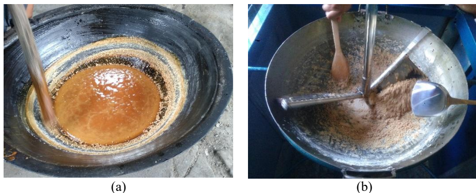
Figure 2. Stirring process during palm sugar granulation: (a) manual stirring; (b) mechanical stirring
