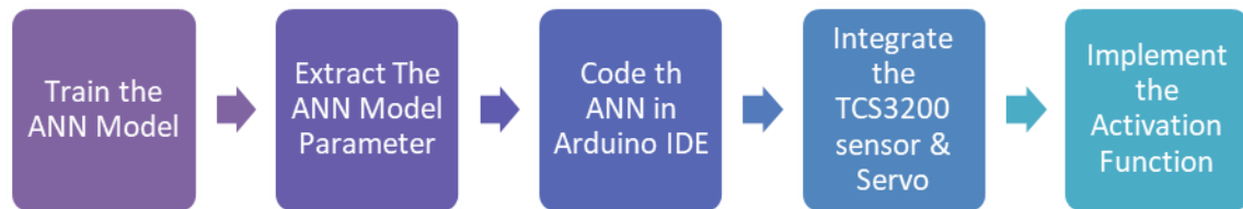
Figure 7. Conversion of the ANN program to Arduino process
