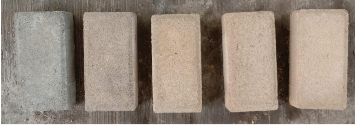
Image 1. The paving blocks that have been molded with the composition (a) P0, (b) P1, (c) P2, (d) P4, and (e) P5.
