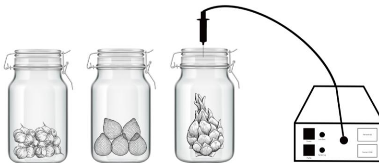
Figure 1. The experimental setup for measuring the respiration of shallots, snake fruit, and dragon fruit
