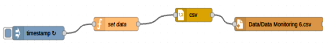
Figure 8. Mechanism of local data recording
