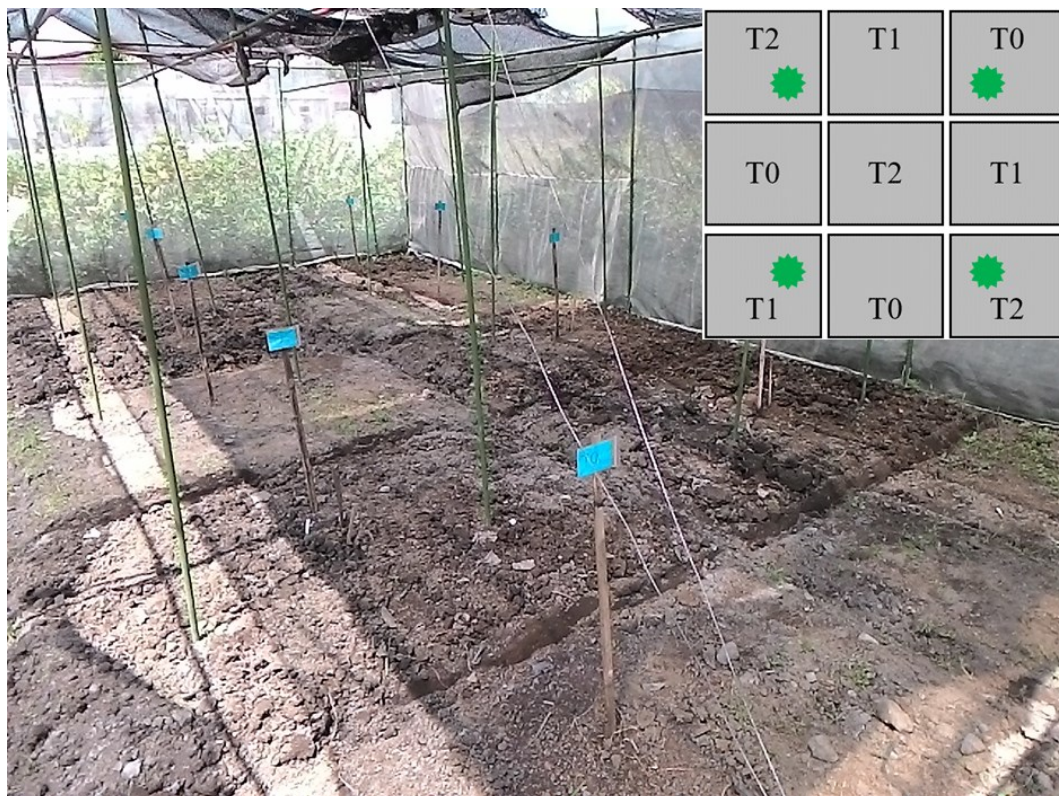
Figure 1. Experimental plot for infiltration experiment. (Inseted: Plot layout and rain discs position represented by green stars)
