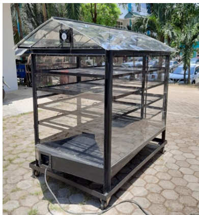
Figure 1. Rack-type hybrid dryer (Warji & Tamrin, 2021)
