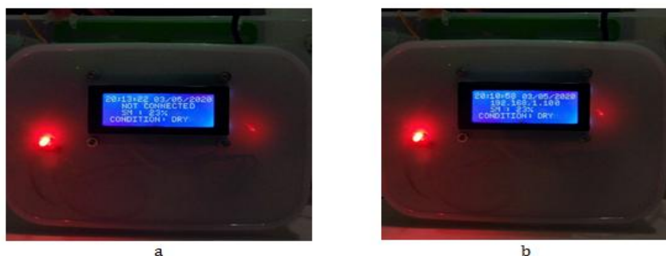
Figure 15. (a) The Information Display is not Connected to The Access Point on The LCD and (b) The Information Display is Connected to The Access Point on The LCD
