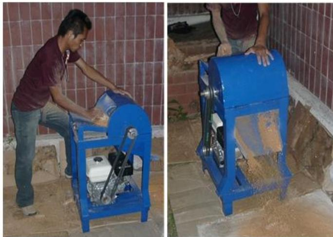
Gambar 3. Cara Pengoperasian Mesin Parut Sagu Tipe Silinder Bertenaga Motor Bakar.
